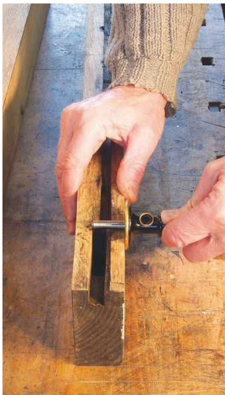
▲ Pic.4 A wheel gauge is expensive but easier to set than a pin gauge
